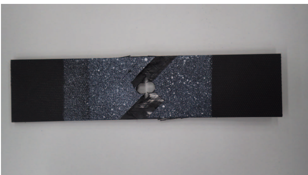
Fig. 6 Specimen After Failure (front)
