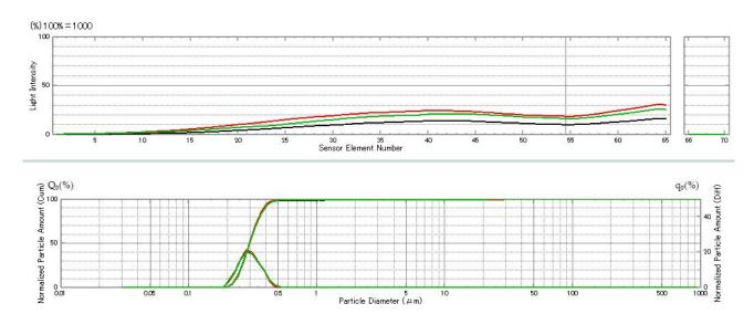
Upper graph shows the light intensity spread over the single detector elements. The lower graph shows the particle size distribution with a peak at 0.4µm.
