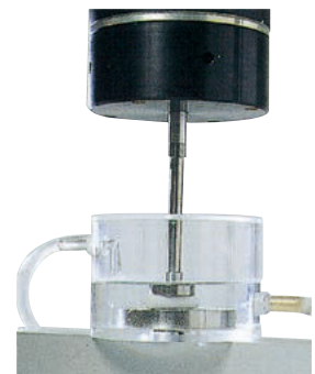
The thermostatic water immersion test unit is ideal for testing biological material and implants.
