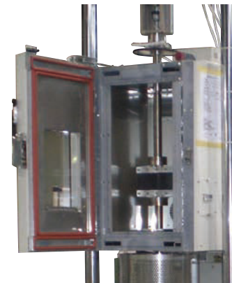
Due to the large testing space, tests can be performed inside a thermostatic chamber.
