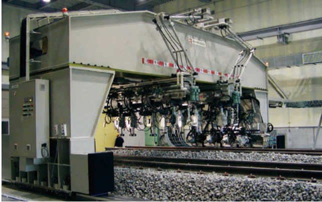
Multiple Jack System on the Railway Rail System Installed for East Japan Railway Company
