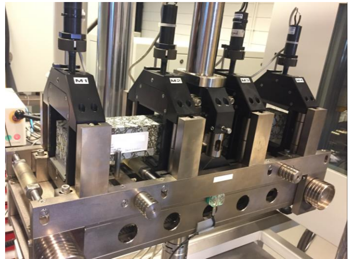
Figure 2: Assembly for 4PB Stiffness test
